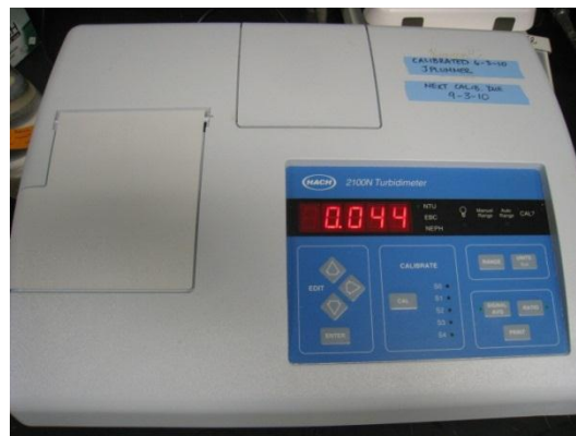
Figure 4.1 Showing Hach 2100N Turbidimeter
