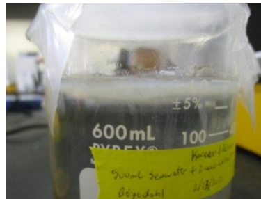
Figure: 24 Emulsion formed first with 500mL seawater and 2.0mL of COREXIT followed by the addition of 0.0394 inch sand
