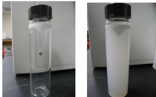
Figure 4.2 Illustrates Empty and fill vials used to test for Turbidity in Hach 2100N Turbidimeter
