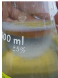
Figure: 14 Emulsion first 500mL seawater + 1.5mL of COREXIT + 0.0029 inch sand
