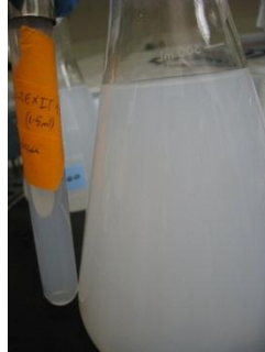
Figure 1 Side view of 500mL of pure water mixed with 1.5mL of COREXIT 9500A
