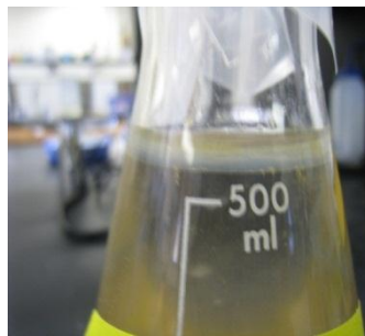
Figure: 20 Emulsion formed first with 500mL seawater and 2.0mL of COREXIT followed by the addition of 0.0029 inch sand
