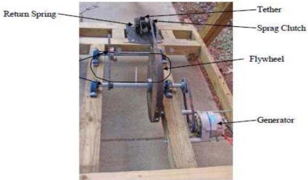
Figure 4: Generator and Flywheel on WPI Kite System
