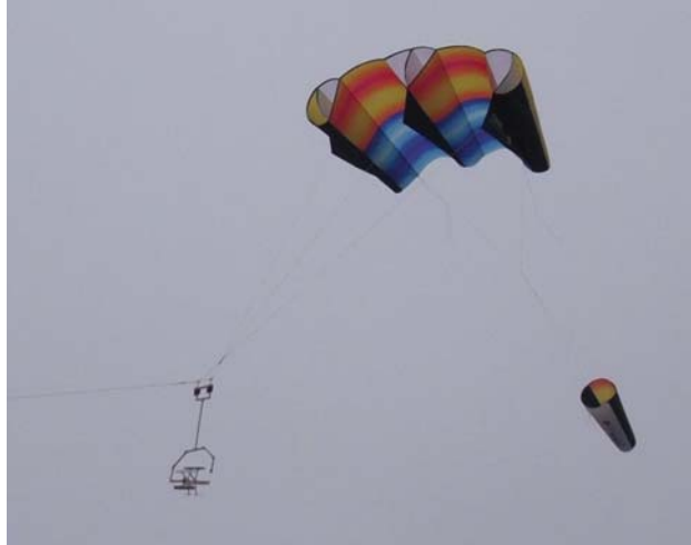
Figure 49: Kite Successfully Lifting Support Frame and Turbine
