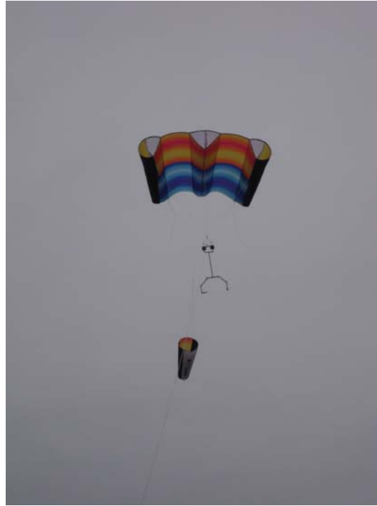
Figure 48: Kite with Turbine Support Frame, Note Roll of Frame
