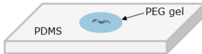
Figure 8: Simple schematic of PDMS stretching apparatus with glued hydrogel embedded with an animal
