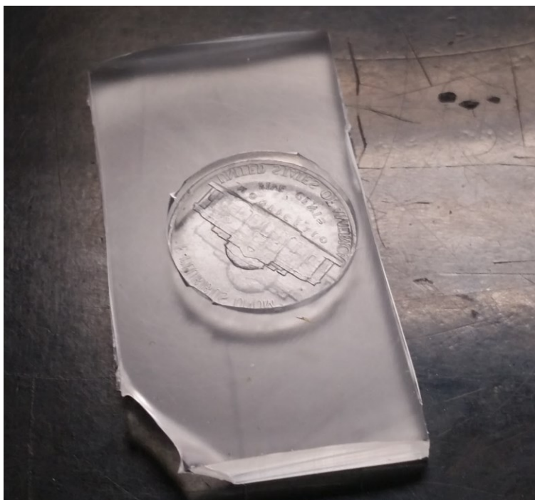
Figure 14: Image of PDMS slab with a hydration well
