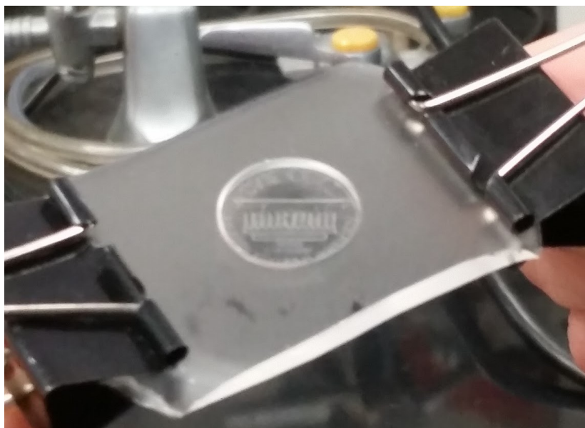
Figure 15: PDMS slab with gripping binder clips to attach to linear actuator
