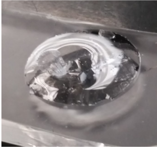
Figure 16: PDMS with hydrogel successfully attached and hydration well filled
