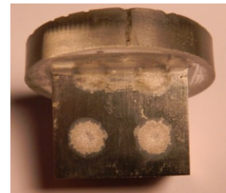
Figure 3: OES sample points (round discolorations) on a specimen that has been partially mounted in epoxy.
