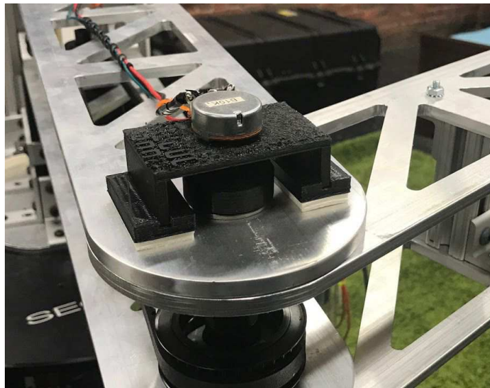
Figure 7G: Picture of potentiometer mount on second joint
