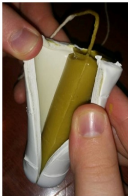
This candle was made from a silicone caulking material mold. The simple mold was created using the listed procedure.
