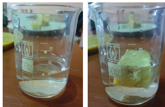
Figure 4.26 (left): Displacement method before (Cane et al.)
