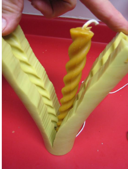
Figure 2.13: Rubber Silicone Molds (Shaw, 2013)
