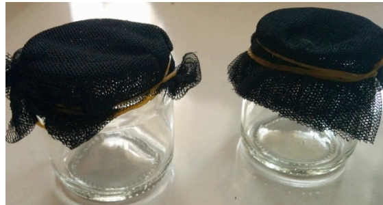
Figure 4.3: Layered chiffon filters (Cane et al., 2014)
