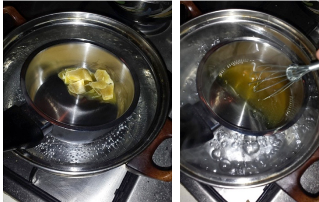
Figure 4.24 (left): Melting beeswax and almond oil in a double boiler (Cane et al.)
