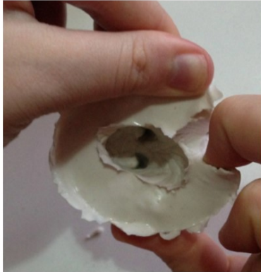
Silicone rubber mold made from listed procedure.
