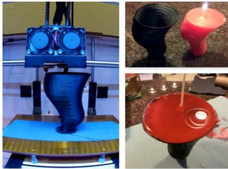
This is how a 3D printed mold is created and filled with wax to create a final candle.
