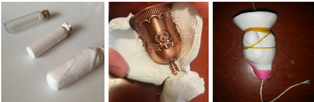
Figure 4.19 (left): Layering with caulking (Cane et al.)
