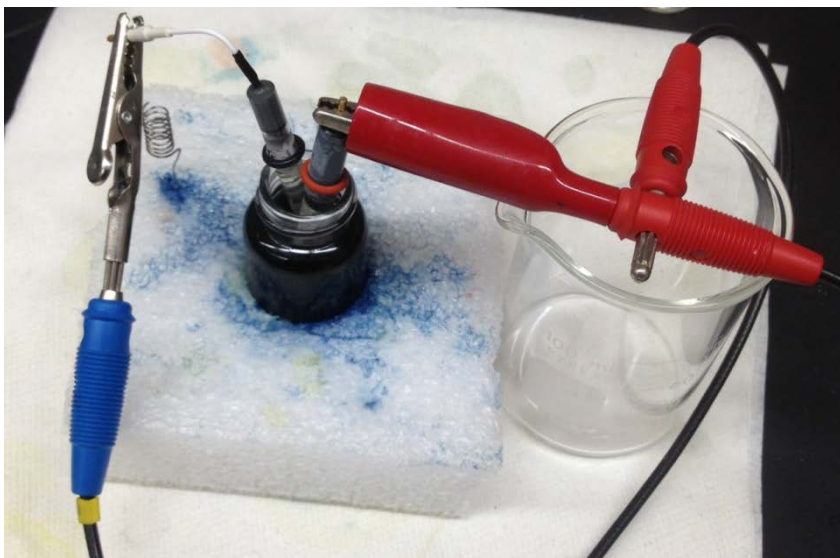
Figure 25: PPy electrochemical film deposition set up
