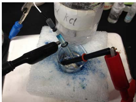
Figure 26: Set up of the lactate amperometry
