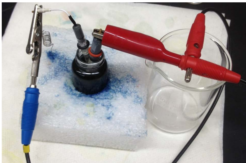
Figure 33: Setting up the biosensor for PPy deposition
