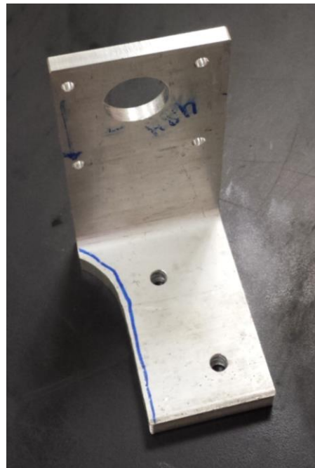
Figure 40: Motor Bracket Prior to Painting
