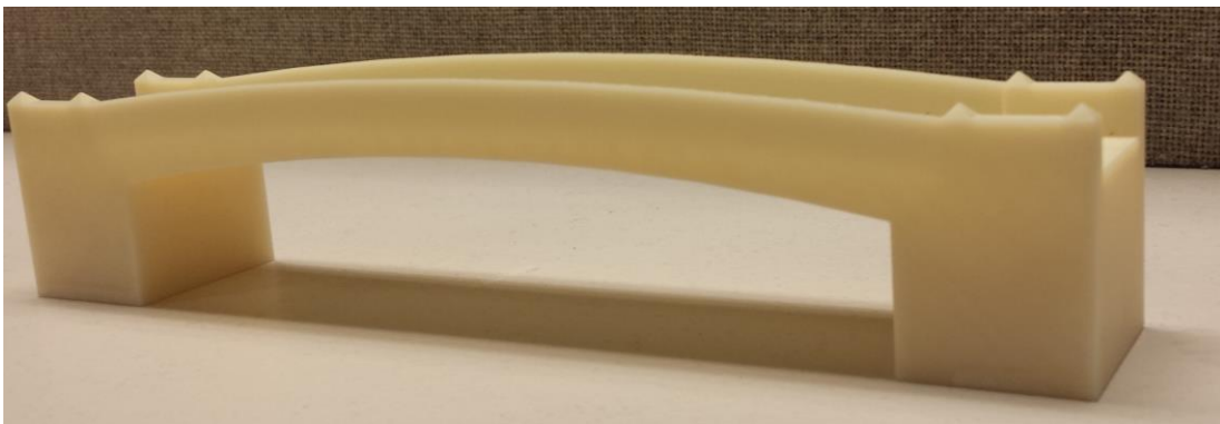
Figure 54: Rapid Prototype of Earle Bridge
