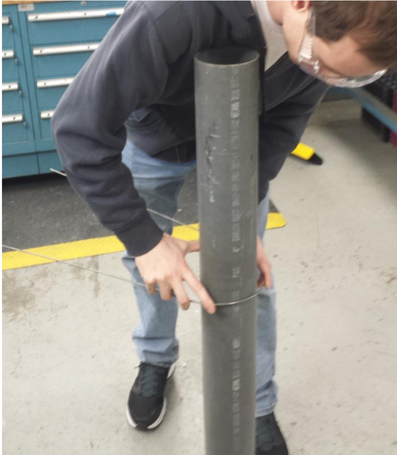
Figure 27: Track Being Bent with a Desired Radius
