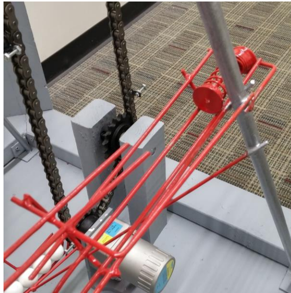
Figure 82: Spring Feeding the Wavy Track Moguls
