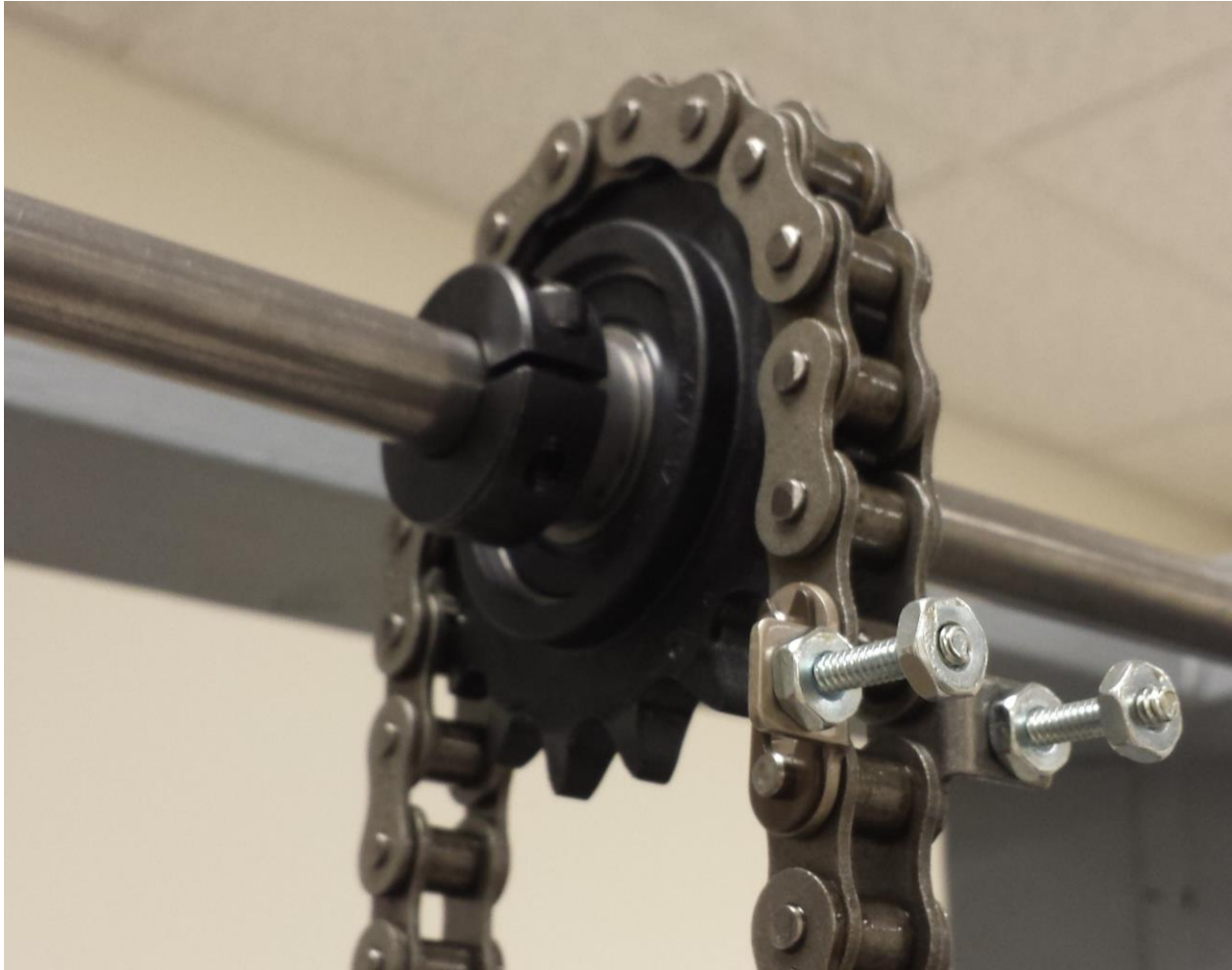
Figure 47: Shaft Collars Located on Top Sprocket
