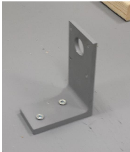
Figure 42: Motor Bracket Secured to Frame
