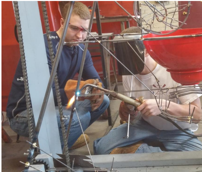
Figure 28: Team Brazing a Section of Track
