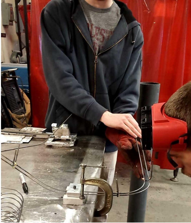
Figure 26: Track Being Bent into Desired Form
