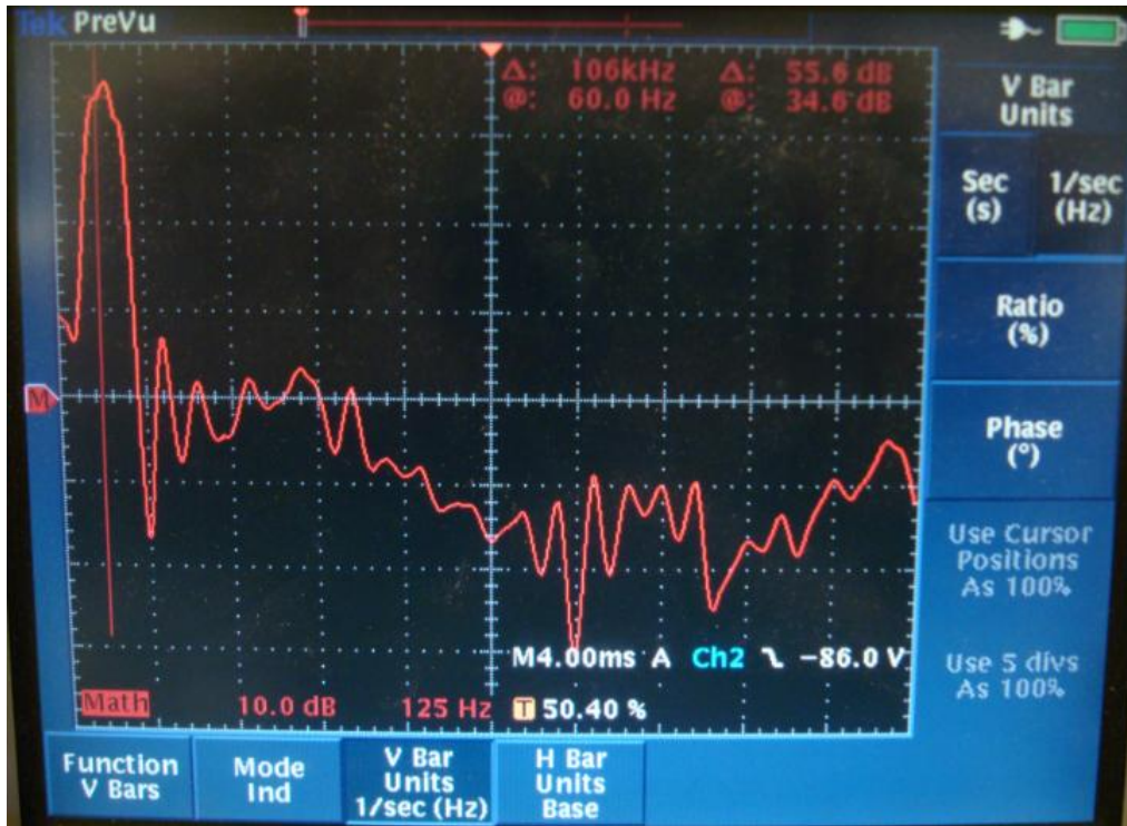
Figure 59: Output FFT showing 60Hz peak
