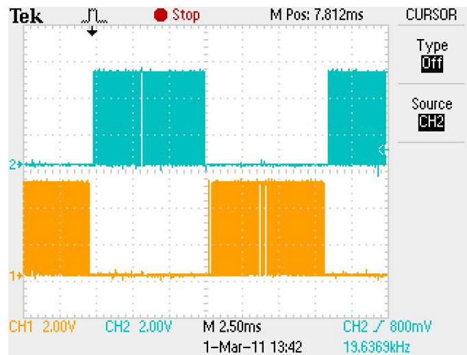
Figure 50: Alternating PWM Signals for Both High Side Gate Half-Cycles
