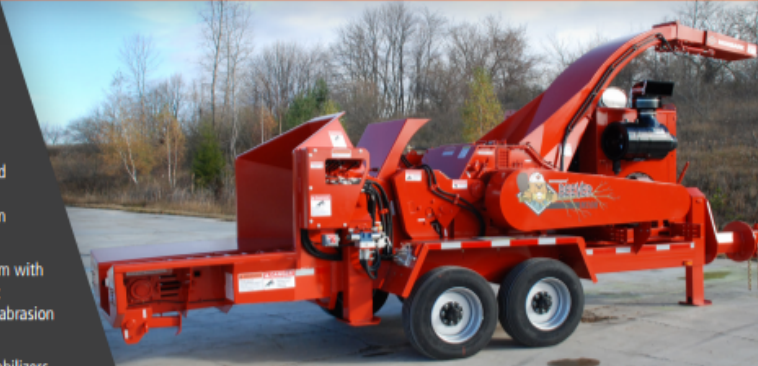
A 6' (1.83 m) infeed bed with live WDH-110 chain drive
