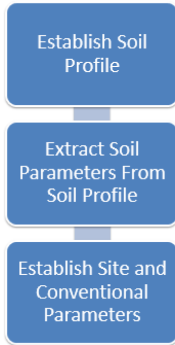
Figure 22: Cantilever Retaining Wall Criteria Flowchart
