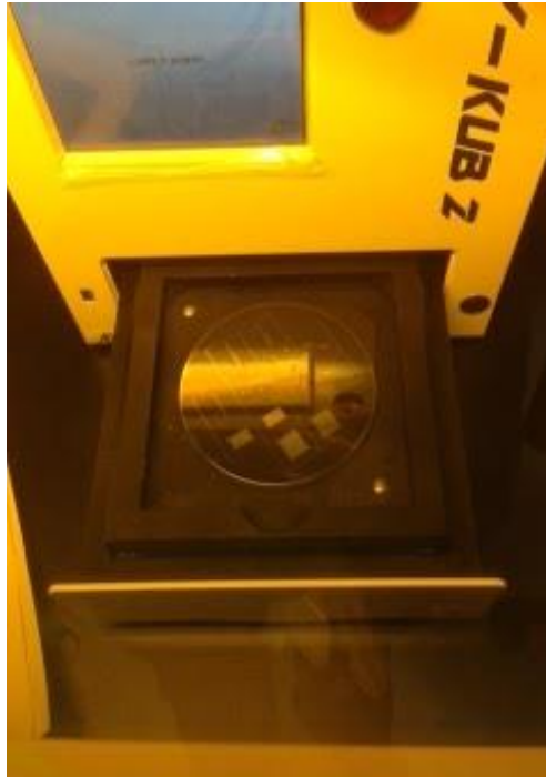
FIGURE 11: SILICON WAFER EXPOSED TO UV LIGHT
