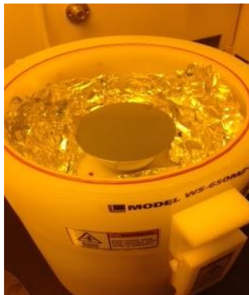
FIGURE 9: SILICON WAFER SPINCOATED WITH PHOTORESIST
