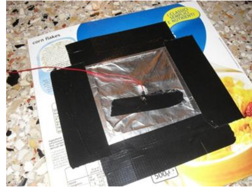
Figure 26: Pressure sensor setup for the "Scents and Sensibilities" installation
