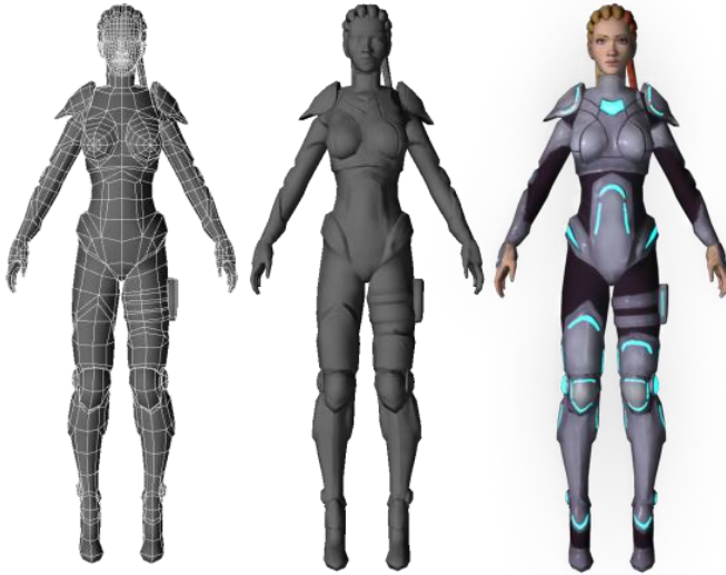
Figure 15: Low-poly game mesh wireframe, low-poly mesh with normal maps, and low-poly mesh with diffuse and normal maps
