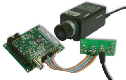
Figure 32. Sensoray Model 311 Frame Grabber with Sample Camera © 2009 SENSORAY EMBEDDED ELECTRONICS. [21]
