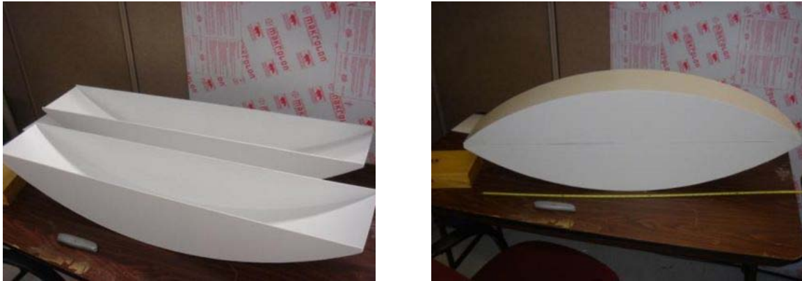
Figure 5. Completed Polystyrene Hull.
