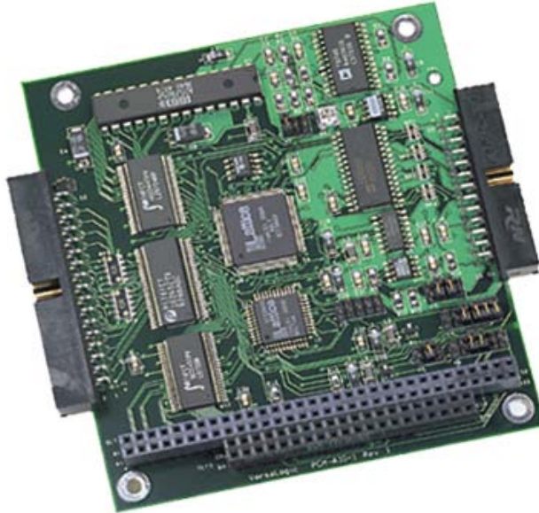
Figure 33. VersaLogic VCM-DAS-1 Data Acquisition and Control Module © 2004-2009 Versallogic Corporation. [24]
