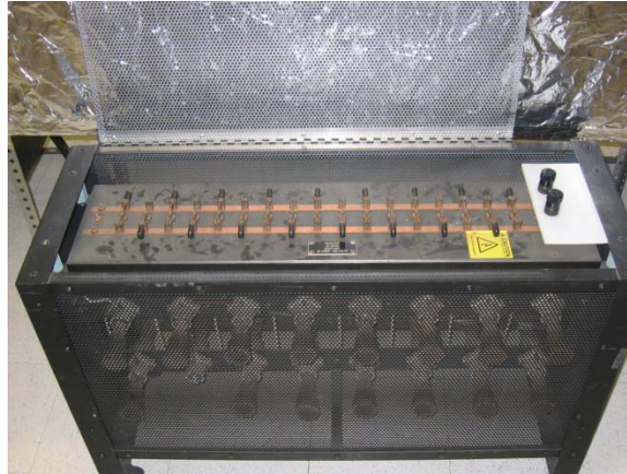
Figure 6. AC Dummy Load Resistor Array.
