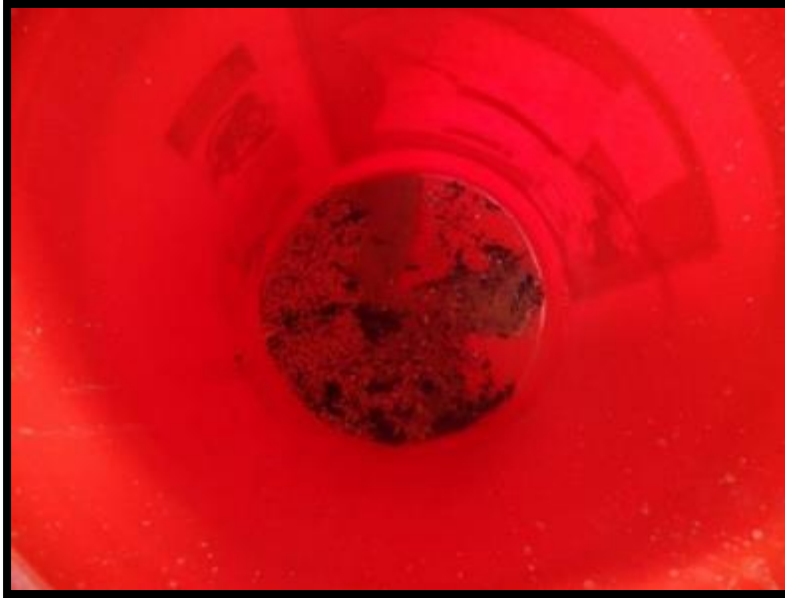
Figure 41. The filter media lost in trial 1 while trying to backwash (media is at the bottom of an orange bucket).
