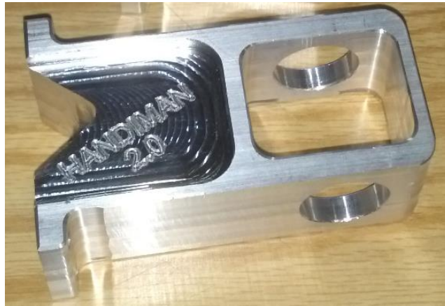
Figure 67-B: Finished Machined Lever Case
