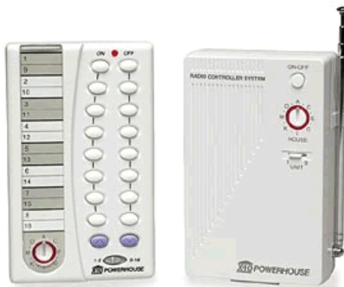
X-10 Controller (left) and Transceiver (right)
