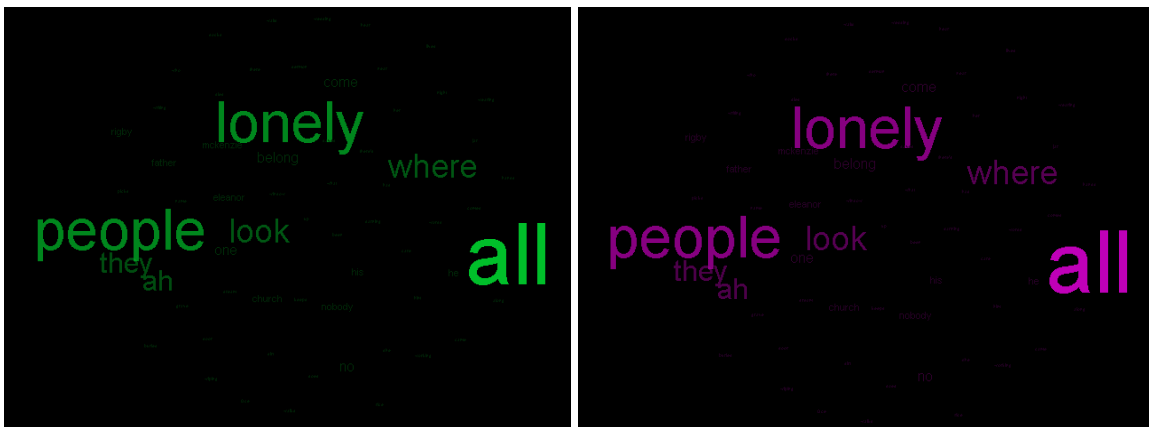
Figure 11: Two screenshots of the DocuCloud with the gradient brightness color scheme, where frequent words – in addition to being drawn larger – are colored brighter in the chosen hue.
