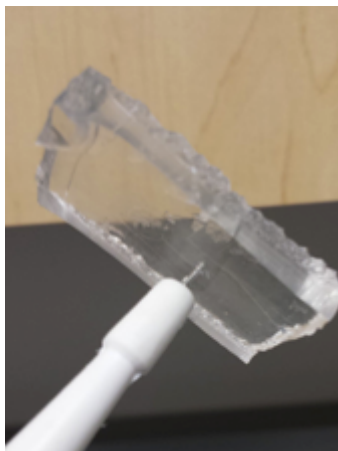
Figure 25 Fabricated PDMS Device with inlet/outlet holes being punched with a biopsy punch
