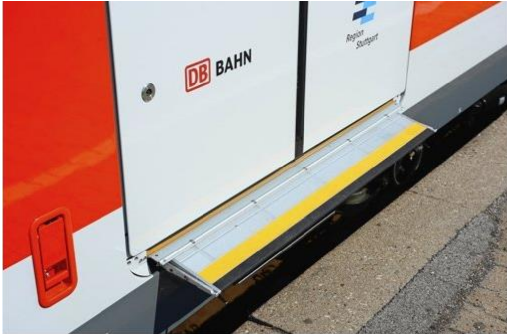
Figure 29. Mechanical Gap Fillers on a German Train Source: (Danza, 2013), without permission
