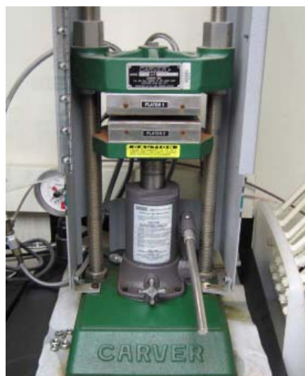
Figure 2.4 GDL is applied to the membrane in the hot press
