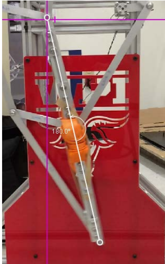
Figure 74: Measured prototype knee angle at maximum extension
