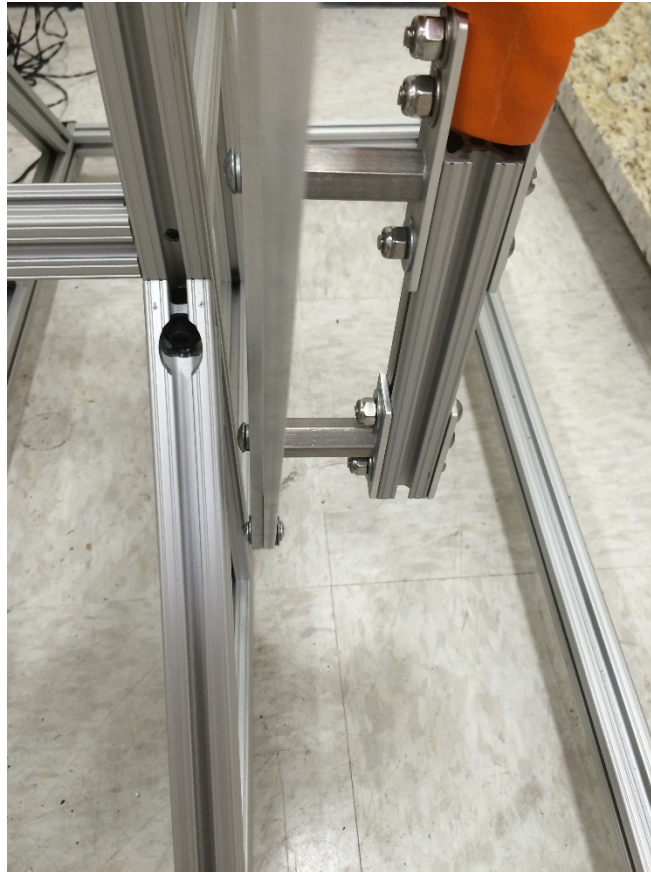
Figure 65: The Bottom Node of the Linkage Impacts the Frame due to a Moment on the Ground Nodes.
