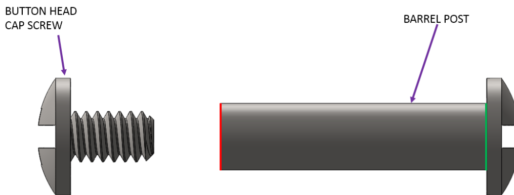
Figure 79: Image of aluminum screw binding post. The red line denotes the flare at the bottom of the barrel near the cap screw and the green line denotes the flare at the top of the barrel post.
