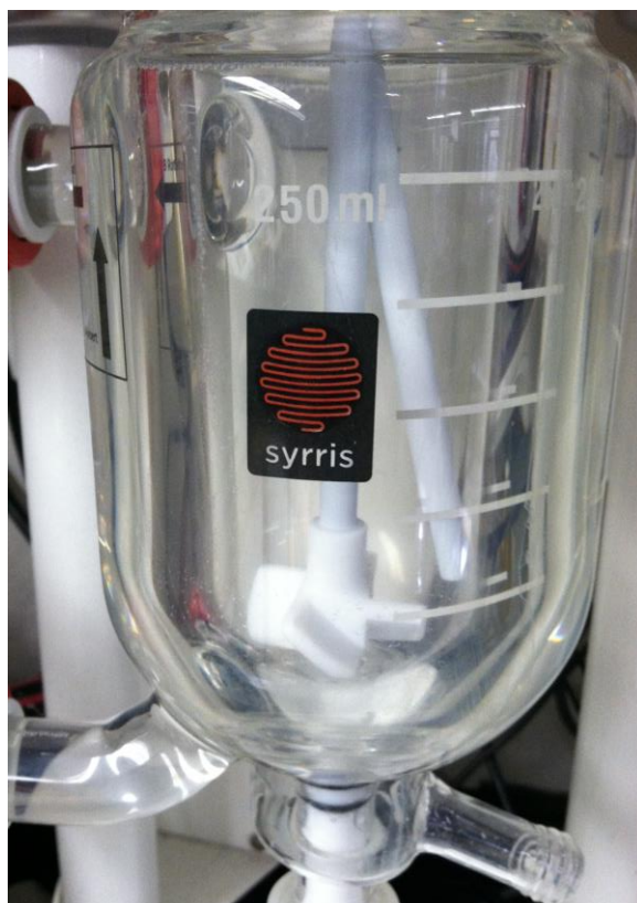
Figure 6: Small reactor with a heating water jacket
