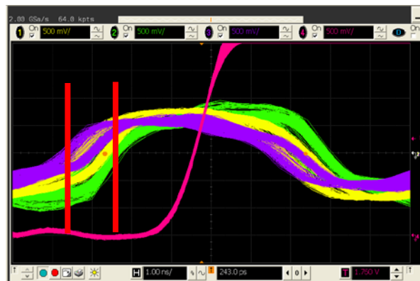
Figure 2: Oscilloscope Test. The 1 PPS trigger is shown as the pink trace; the other three channels (purple, yellow, and green traces) are connected to three USRP2s. After running for 30 minutes, the maximum time offset was less than 2 ns.
