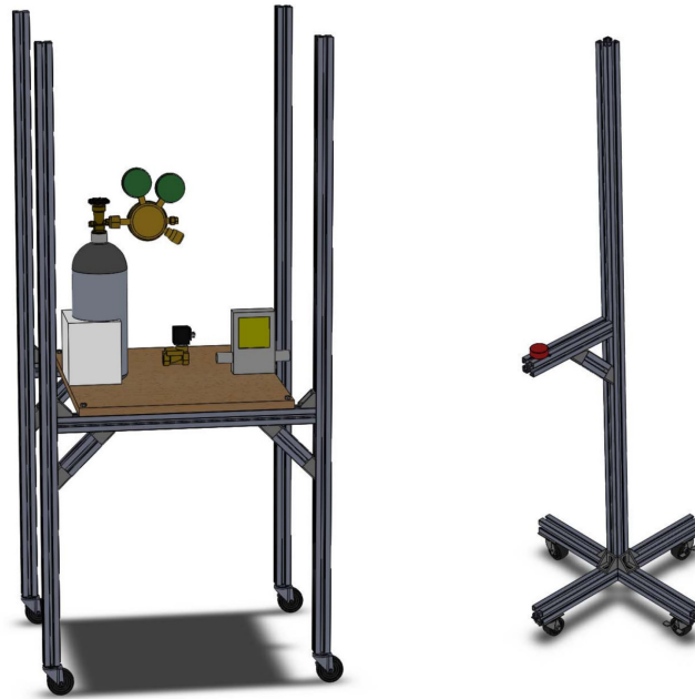
Figure 2.1 Plume Generation (Left) and Plume Detection (Right) Stands.
