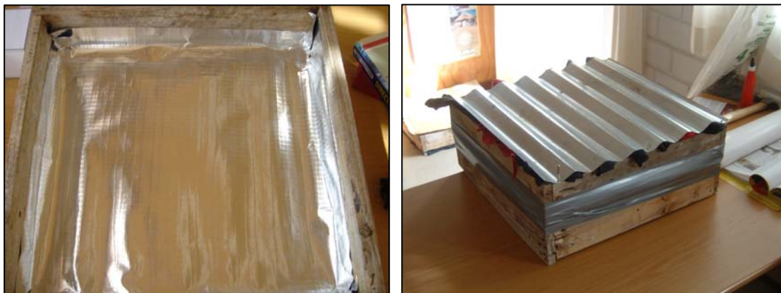
Figure 8: First Sample- Sisilation™ directly underneath (left) and Second Sample- Sisilation™ with an air pocket (right)
