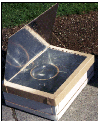
Figure 12: Solar box cooker (left) and Structure of a solar box cooker (right) Source: http://www.exoticblades.com/tamara/sol_cook/types.html (left) and http://www.solarcooking.org/sbcdes2.htm (right)
