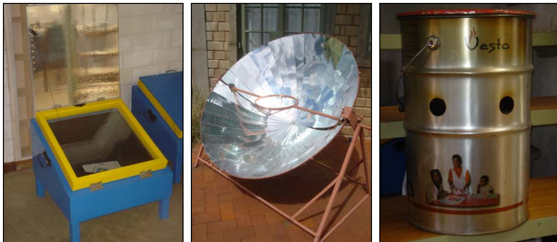
Figure 4: Solar Box Stove (left), Parabolic Solar Cooker (center), and a Vesto (right)
