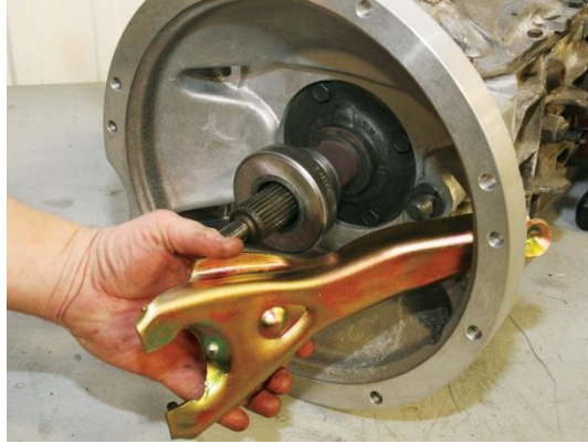
Figure 17 Similar fork found in standard transmissions (Bernsau, 2013)
