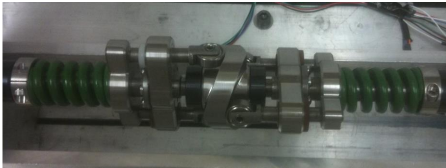
Figure 3 Collins et al's Cam Separation Spring (Collins, 2011)
