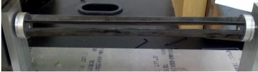
Figure 2 Araujo et al's prototype Torsion Spring (Araujo, 2008)
