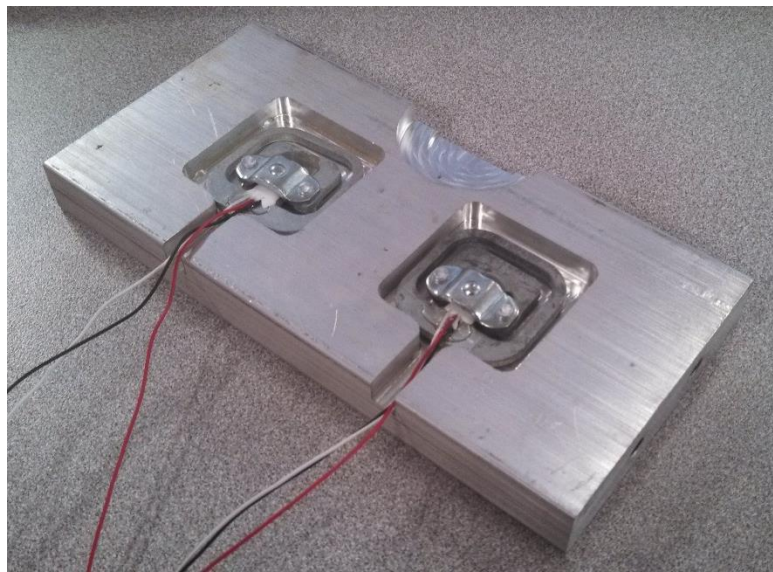
Figure 57-Load cell configuration with nest milled into back stand
