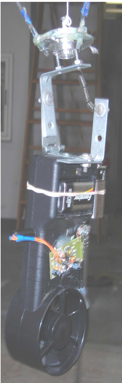
Figure 3.6 - Close up of the anemometer assembly
