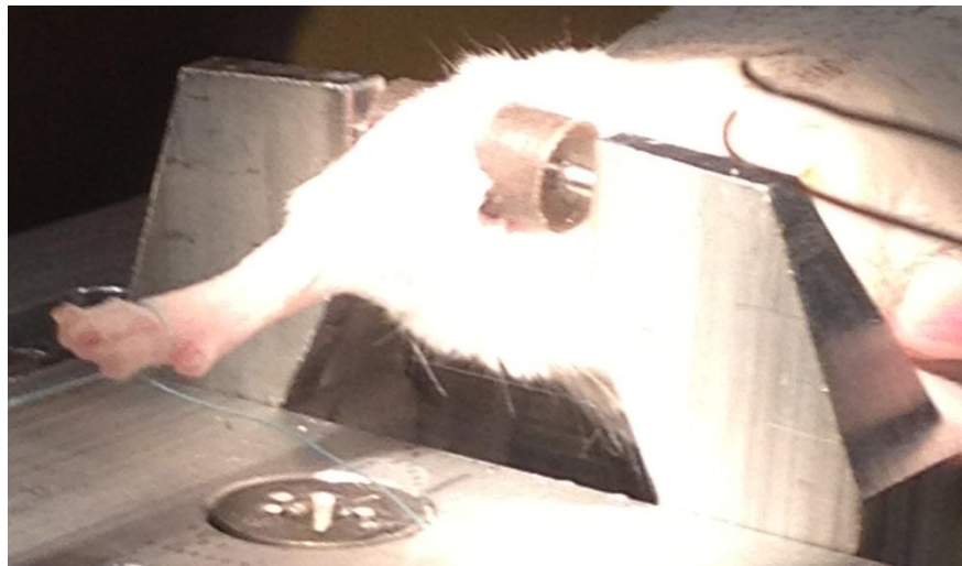
Figure 23: Photo of deceased mouse knee fixated between modular spring-loaded clamps
