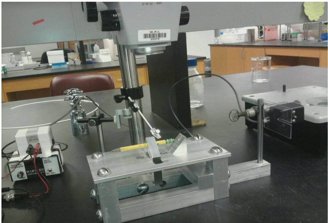
Figure 19: Photograph of initial knee fixation design during preliminary pencil test
