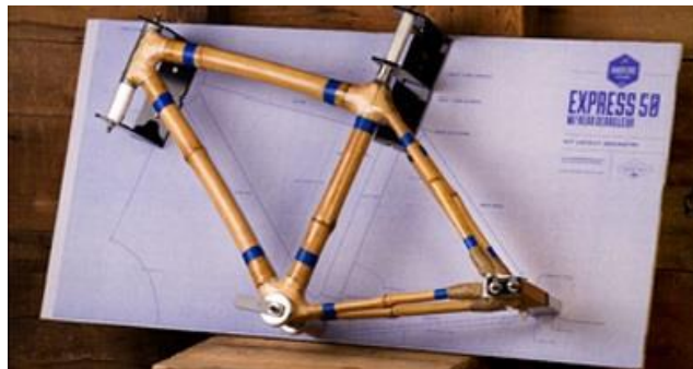
Figure 2. Backing Plate Jig, from HEROBike
