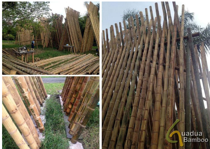
Figure 73. Vertical Drying, from http://www.guaduaibamboo.com/bamboo-poles/
