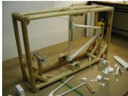
Figure 4. Frame Jig, from http://www.instructables.com/id/How-I-built-a-carbon-bike-frame-at-home-and-a-bam/
