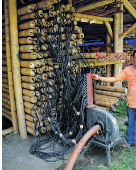
Figure 75. Forced Convection Drying, from (Minke 2012)
