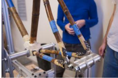
Figure 3. Frame Jig, from https://bamboobike.wordpress.com/other-peoples-projects/
