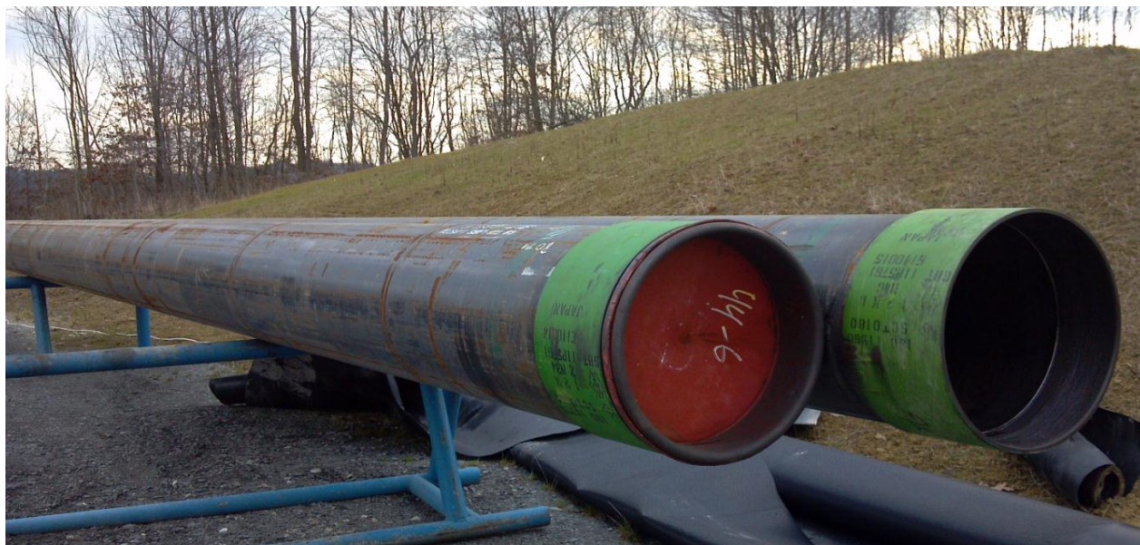
Figure 16: Twenty Inch Surface Casing
