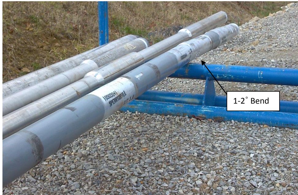
Figure 12: Horizontal Drilling Motor Assembly
