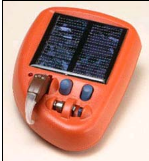
Figure 7: Solar battery charger for hearing aids developed by Godisa 46
