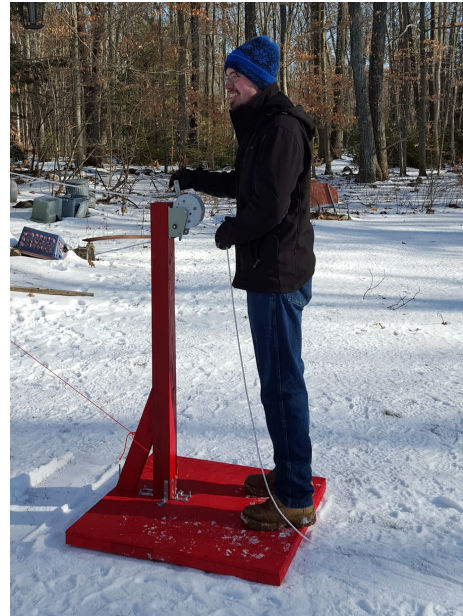
Figure 55: Winching Platform in Action
