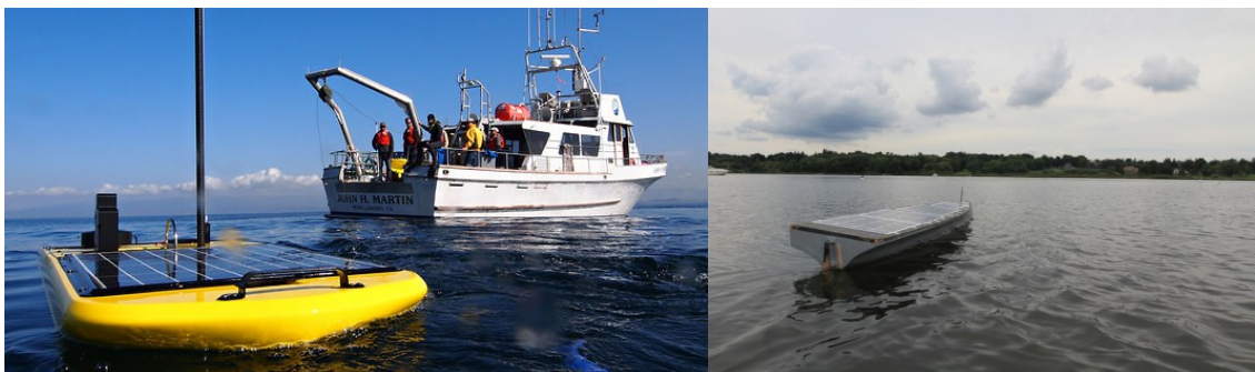
Liquid Robotics' Wave Glider (left) and SCOUT, another long range ASV (right).
