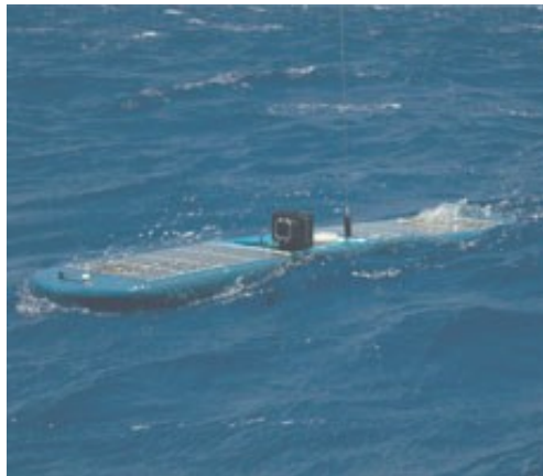
Figure 8: SHARC Wave Glider- the company's defense oriented ASV unit (Liquid Robotics, 2012).
