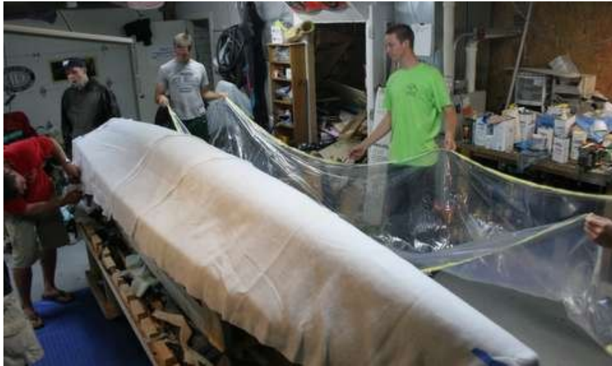
Figure 11: SCOUT construction using a vacuum lamination technique to apply carbon fiber to the bottom of the hull (Rodriguez, 2012).
