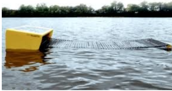
Figure7: Seaswarm prototype showing the belt propulsion (Senseable Sea Labs, 2012).
