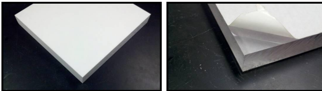
Figure 26. Ultra-high molecular weight polyethylene (left) and polycarbonate (right)
