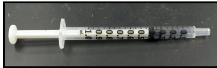
Figure 28. 1 mL push-connect or luer-slip syringe
