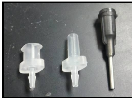
Figure 21. Pictured left to right, 1/16" inner diameter female barbed luer-lock tip, 1/16" inner diameter male barbed bayonet tip, and 2mm blunt end metal syringe tip.
