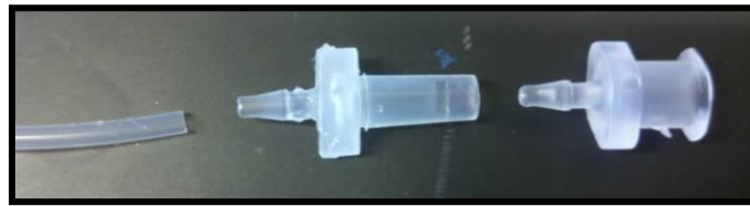
Figure 22. Syringe-silicone tubing connectors
