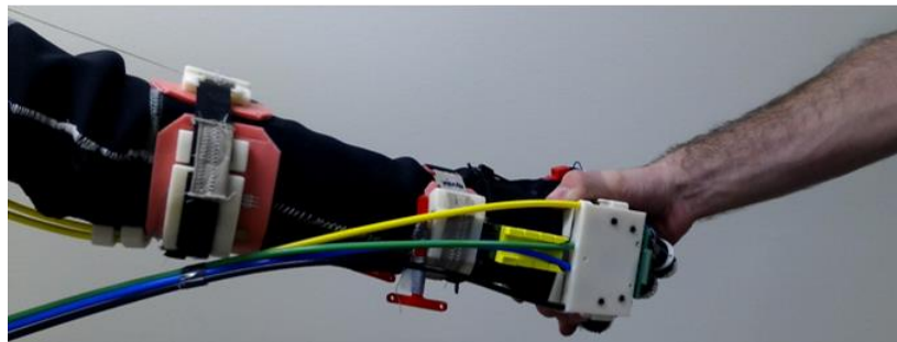
Figure E: Exomuscular Sleeve Final Prototype.
