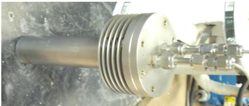
Figure 63: Steel Vessel for Sparger and potential Cold Trap Usage
