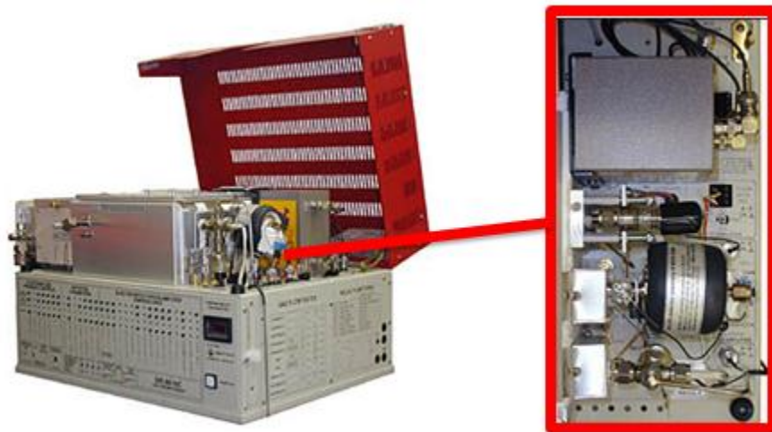
Fig. 31: The SRI 8610 Gas Chromatograph (TCD Detector shown as the grey box in the top right of the image)
