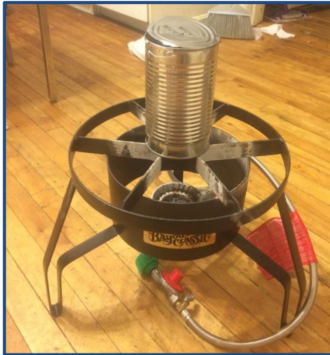
Figure 16: Heat Source – Propane Burner
