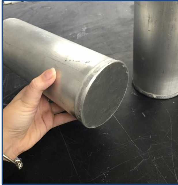
Figure 26: Welded Cylinder Cap
