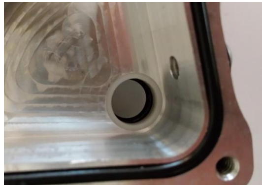
Figure 30: Delrin acetal resin bushing firmly in place within case half housing
