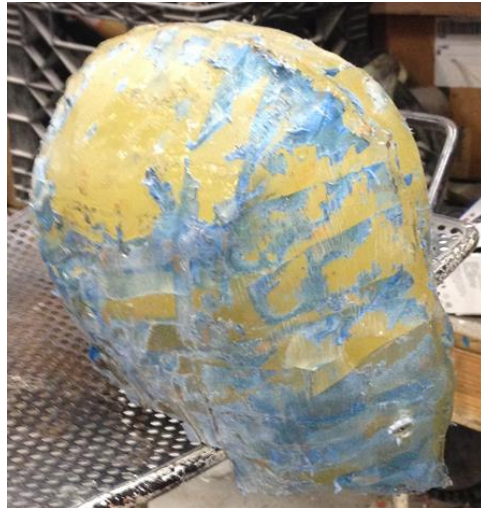
Figure 47: Epoxy head prior to final cleaning
