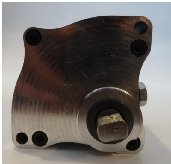
Figure 32: Steel shaft through rubber seal on assembled device
