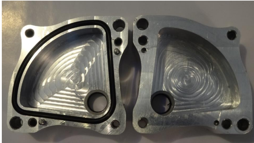
Figure 26: O-ring in groove on left, flat surface on right
