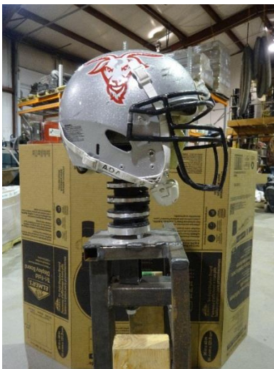
Figure 50: Neck/Torso Assembly with Cable Tensioner
