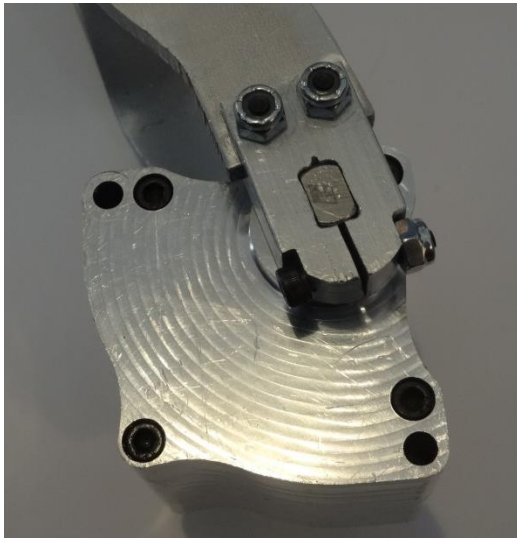
Figure 36: Clamp tightly fastened to steel shaft
