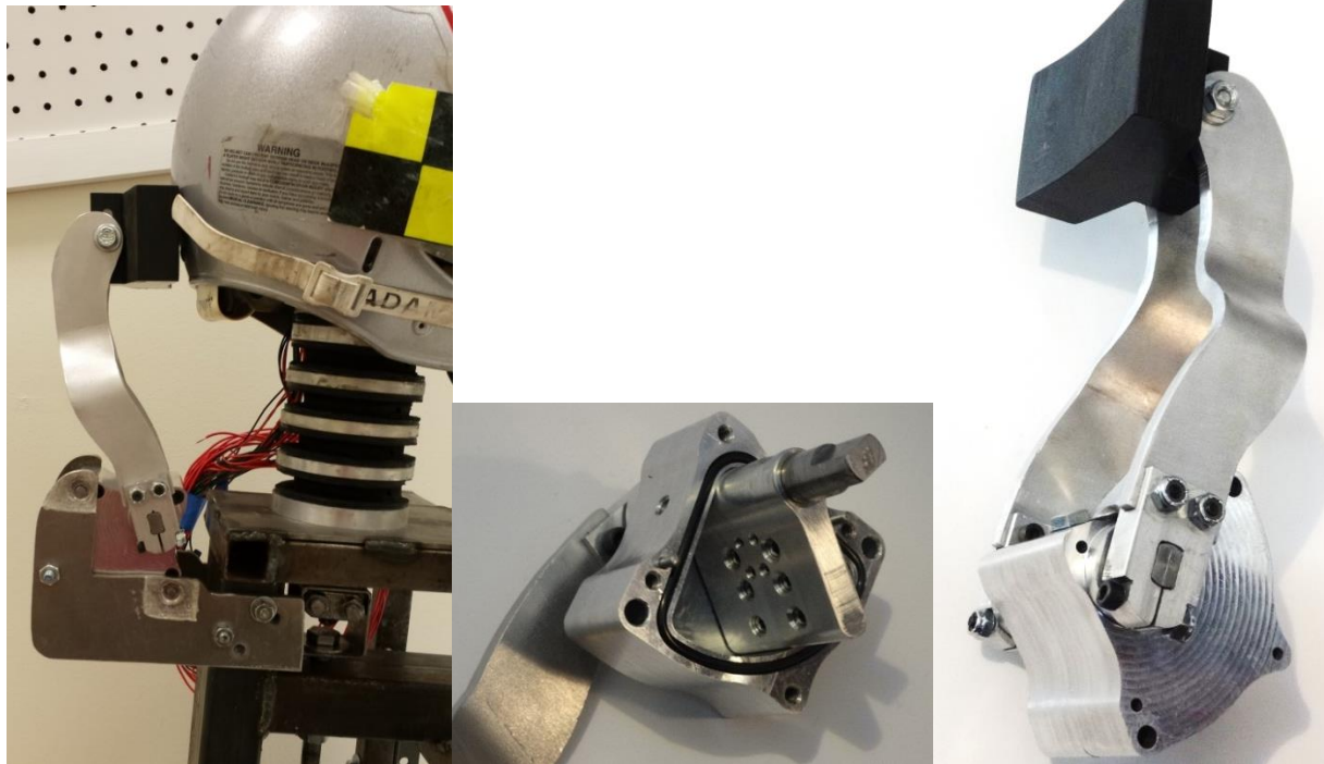
Figure 4: Manufactured rotational shock absorber. Left on torso supporting helmet. Middle casing half open to show paddle with holes. Right fully assembled device
