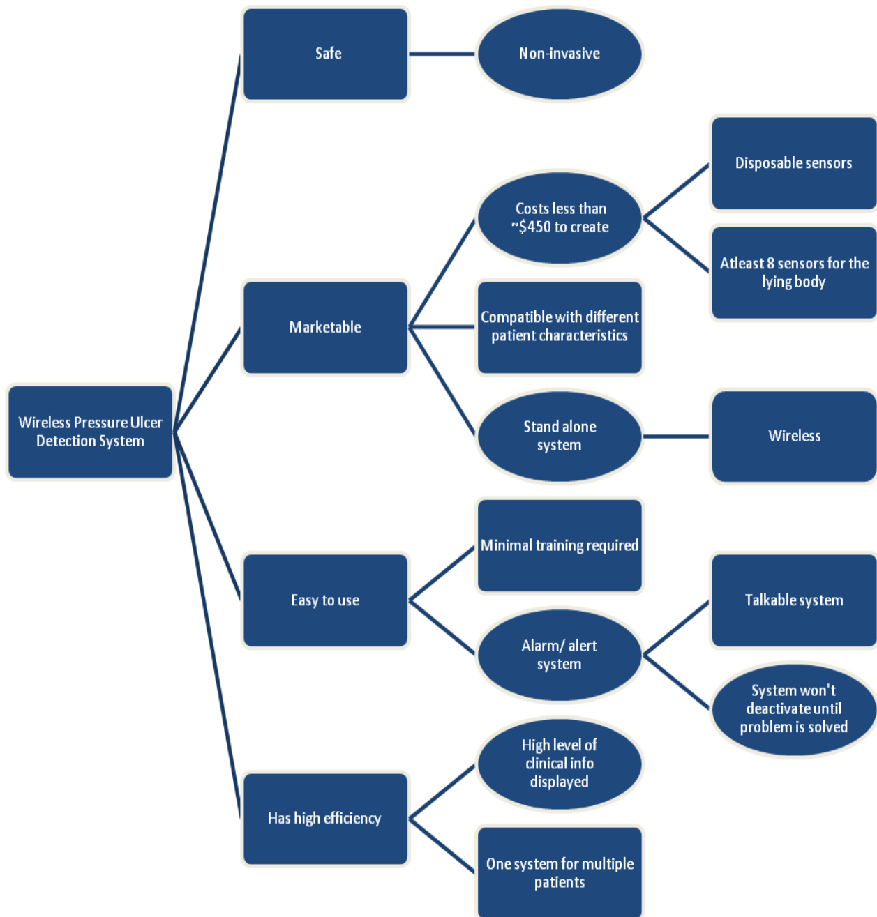
Figure 10: Combined Objectives and Constraints Tree.
