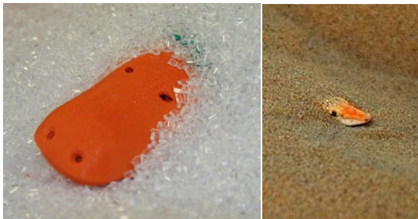
Figure 43: The Snake Robot in the Testing Bed and a Real Snake in the Desert
