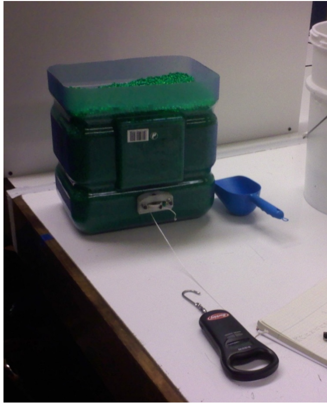
Figure 12: Torque Testing Experimental Setup
