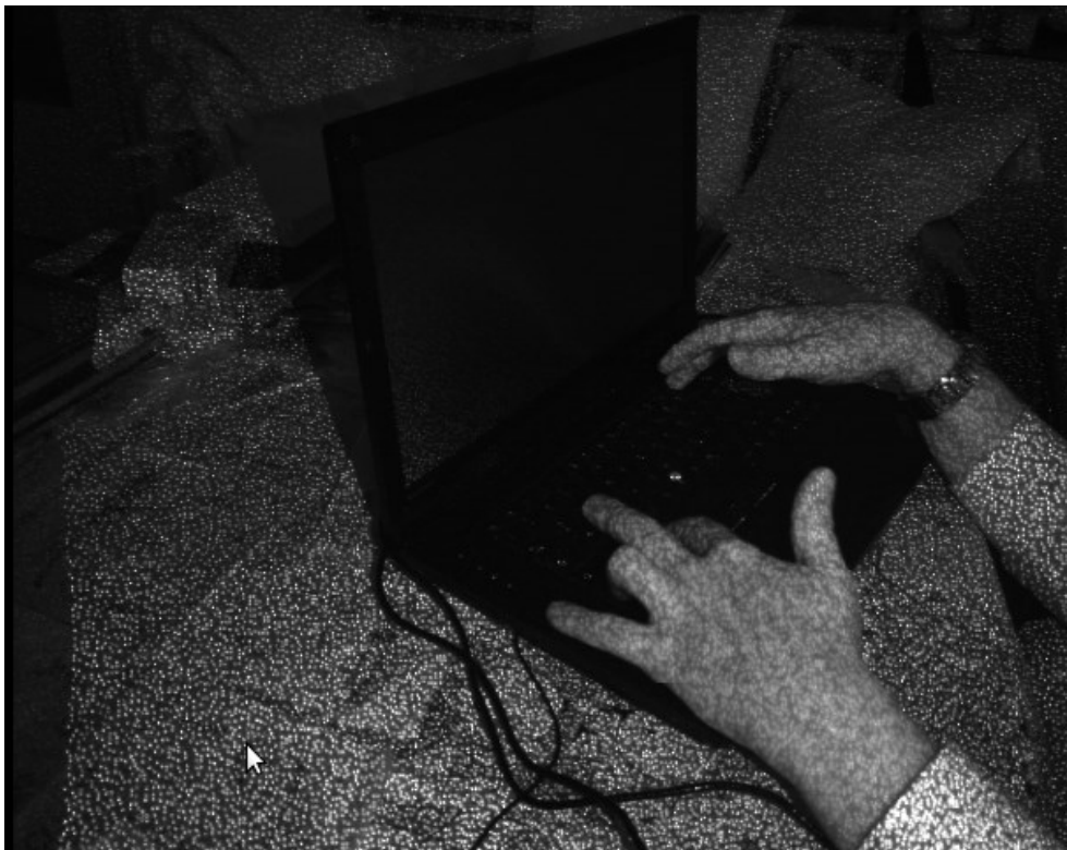
Figure : Microsoft Kinect IR Projection [5]
