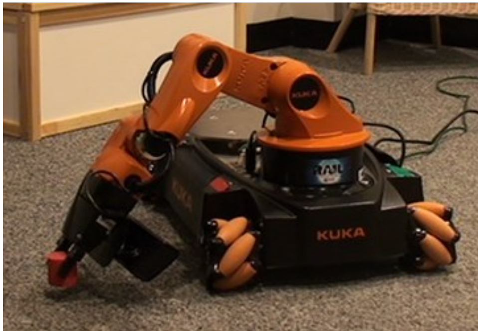
Figure : The youBot picking up a cylindrical block with an angled grasp
