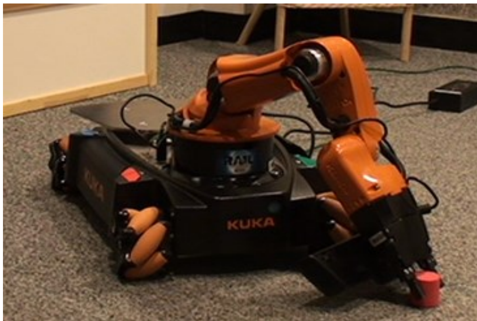
Figure : The youBot placing a cylindrical object that was picked up with an angled grasp
