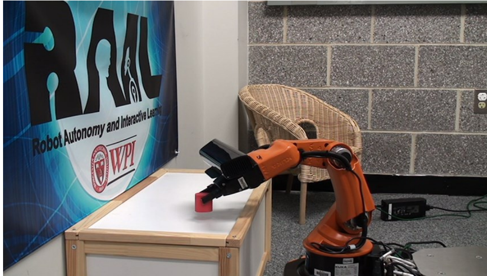
Figure : The youBot picking up a block off a table
