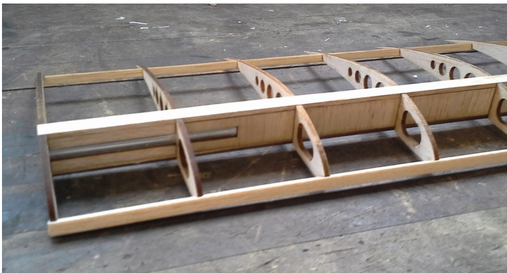
Figure 25-Internal structure of the load-to-failure test wing
