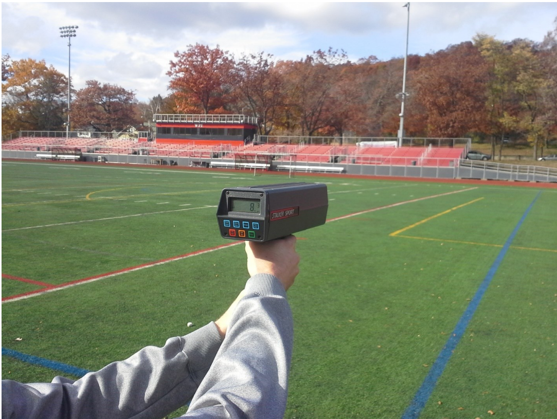
Figure 13-The radar gun used to measure expected launch velocity.
