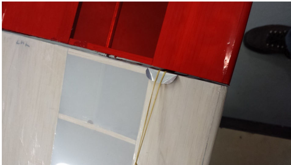
Figure 32-Flying wire wing attachment
