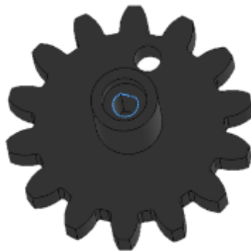
Figure 35: Driving gear with highlighted D-profile hole for motor shaft entry
