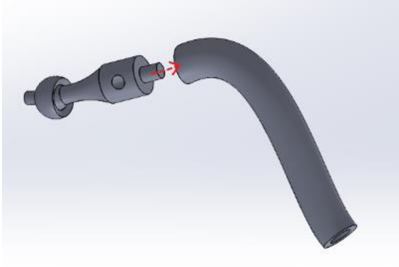
Figure 32: Connection achieved using adhesives, by assembling in the position of the red arrow. The ball-socket joint is on the left, connecting to the lower leg on the right.
