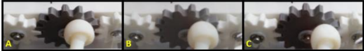
Figure 22: Comparison of (A) leg start location, (B) position after one rotation, and (C) position after two rotations
