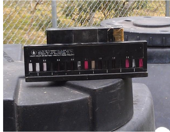
Figure 6: Chloroscope used by Miguel Bertozzi to check residual chlorine during maintenance
