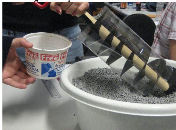
Figure 4: Paper Archimedes Screw
