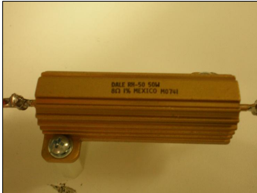
Figure 6.5 Test Load Resistor
