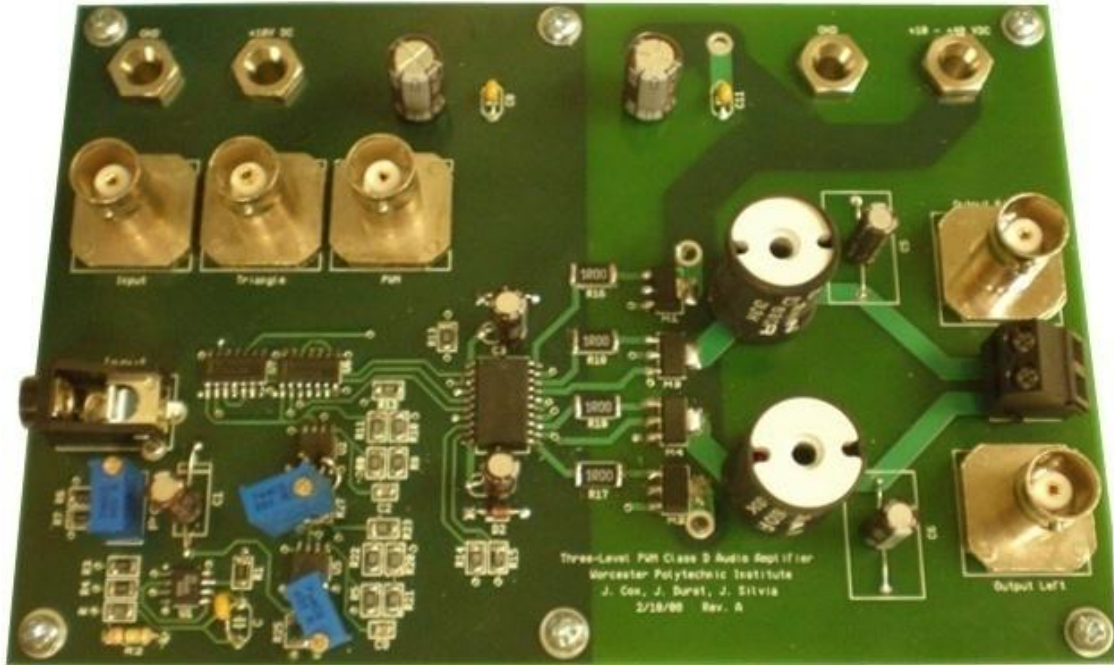
Figure 5.30 Three-level PCB Assembled (Top)
