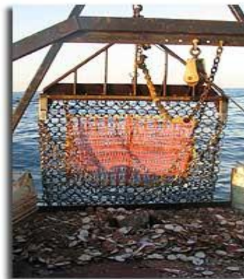
Figure 7: Hauling the dredge onto the vessel (Ruhle, 2007)
