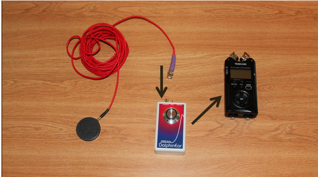
Figure 3. DolphinEar DE200 Series Hydrophone Setup
