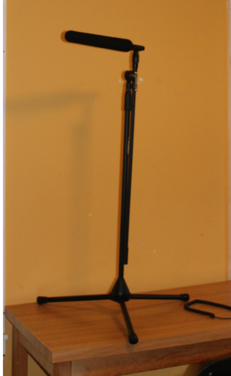
Figure 2. Microphone Stand for Audio-Technica BP4027 Shotgun Stereo Microphone
